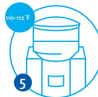
**EN** For machine feeding set the mixing temperature at 110-112°F.
